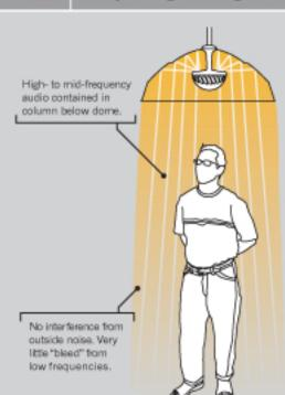
SoundTube FP series speakers achieve remarkable intelligibility by incorporating Dual-Parabolic" dome technology, which provides a dramatic hot-spot with crisp stereo separation. This proprietary technology reflects sound waves from the upper registers of the frequency spectrum directly beneath the dome
